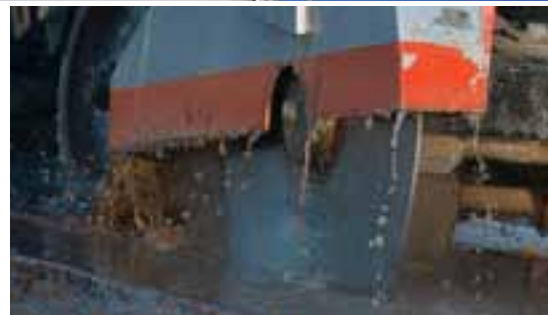
Asphalt blades incorporate hardened steel core to significantly reduce overall blade wear.
